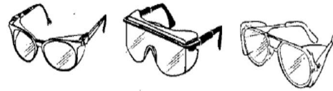
Class 1A - Spectacle-type with side protection
