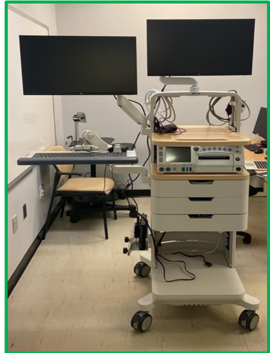
Real Image: Fetal Mobile Cart with a GE Fetal Monitor and PC related hardware mounted. CE and UPS to be installed (WIP)
