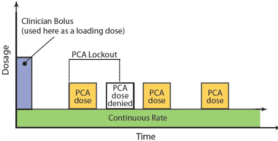
Example 2: Intermittent Boluses (IB) and PCA Doses, with Bolus Interval Type set as PCA Lockout
