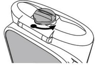
2. Hold the pump at an angle and place 4 AA batteries in the pump, from the bottom up (see picture). Match the + and - markings on the new batteries with the markings on the pump.
