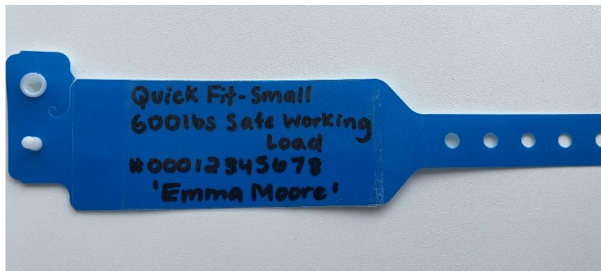
Figure 1: Example of a tag added onto sling. Adding the resident's name is optional.
